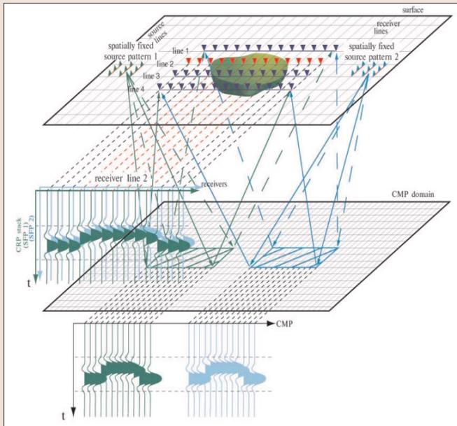
**Figure 3.** Example of how two spatially fixed source patterns “illuminate” a near-surface heterogeneity.
