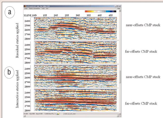
**Figure 7.** Comparison between CMP partial-offset stacks after autostatics (a) and after interactive statics (b).
