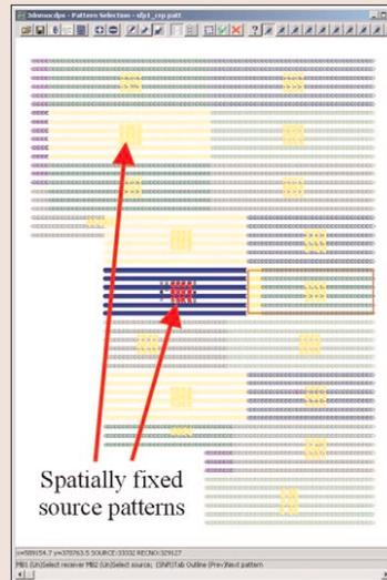
**Figure 4.** A survey map of spatially fixed source groups. Receiver groups, illuminated from differently fixed source groups are shown in different colors.
