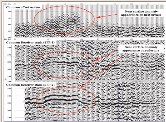
**Figure 5.** Multipanel display of three sections: common-offset (top), CRP SFP set 1 (middle) and CRP SFP set 2 (bottom). The surface-consistent sections are positioned by receivers. The anomaly image remains stationary.
