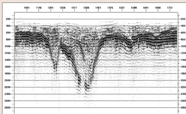
Figure 2. Example of the appearance of surface anomaly on a common-offset time section.
