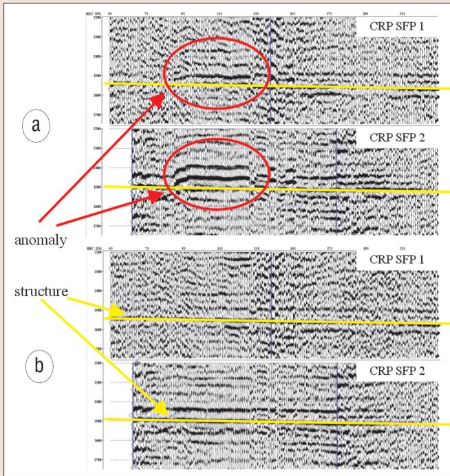
**Figure 10.** Two CRP sections with residual statics applied (a) and interactive and residual statics applied (b).
