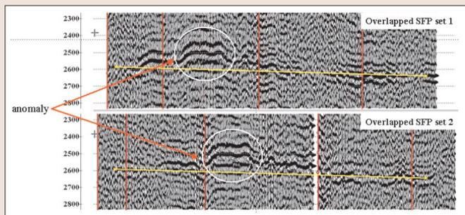
**Figure 6.** CMP-matching. CRP SFP set 1 (top) and CRP SFP set 2 (bottom). Stacks are positioned by CMPs. The anomaly image shifts on the surface consistent stacks.
