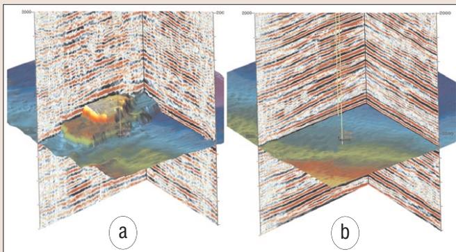
Figure 13. 3D data example of heterogeneous permafrost. Two perpendicular cross sections and horizon time surface. Residual statics applied (a) and interactive statics applied (b).
