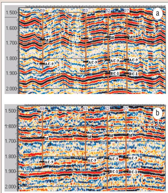
Figure 14. 2D data example of heterogeneous permafrost. Before (a) and after (b) interactive statics.
