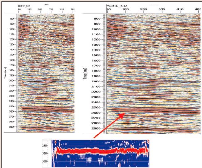
Figure 12. Same data as in Figure 8 after interactive statics.
