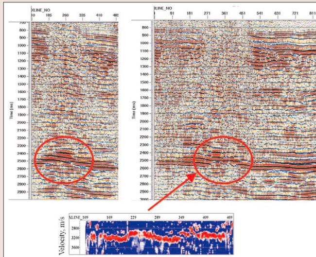
**Figure 8.** Two perpendicular vertical sections (above) and the horizon velocity analysis panel (below). Automatic statics applied.
