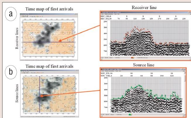
Figure 1. Common-offset sections (right) and first breaks time maps (left) derived from first breaks analysis over all receiver (a) and source (b) lines.
