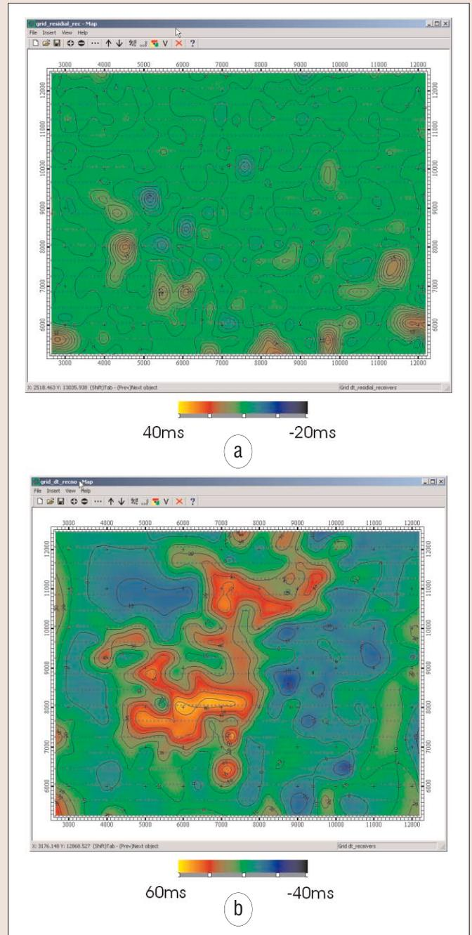
**Figure 11.** Receiver statics time delays after residual statics (a) and interactive statics (b).
